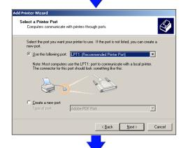
Select the correct port you plan to use, usually the LPT1 (Parallel) port or COM1 (Serial) port.
